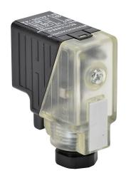
Murrelektronik field wireable solenoid valve connector, 11mm DIN style molded connector, 24 VAC/VDC, 16-12 AWG, accepts cable diameter size 0.24-0.32in, surge protection, LED indication.
