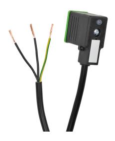
Murrelektronik solenoid valve cable, 11mm DIN style molded connector to 3-wire pigtail, 110 VAC/VDC, 18 AWG, PVC jacket, 16.4ft/5m cable length, surge protection, LED indication.
