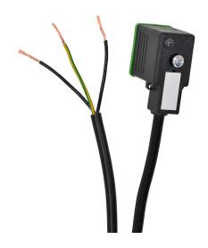
Murrelektronik solenoid valve cable, 11mm reverse DIN style molded connector to 3-wire pigtail, 110 VAC/VDC, 18 AWG, PVC jacket, 16.4ft/5m cable length, surge protection, LED indication.
