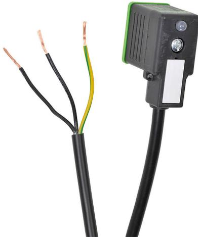
Murrelektronik solenoid valve cable, 11mm DIN style molded connector to 3-wire pigtail, 110 VAC/VDC, 18 AWG, PVC jacket, 9.8ft/3m cable length, surge protection, LED indication.
