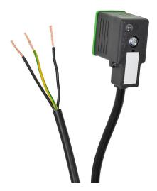
Murrelektronik solenoid valve cable, 11mm reverse DIN style molded connector to 3-wire pigtail, 110 VAC/VDC, 18 AWG, PVC jacket, 9.8ft/3m cable length, surge protection, LED indication.
