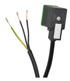
Murrelektronik solenoid valve cable, 11mm DIN style molded connector to 3-wire pigtail, 230 VAC/VDC, 18 AWG, PVC jacket, 9.8ft/3m cable length.
