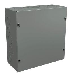
Wiegmann enclosure, NEMA 1,  $10 \times 10 \times 4$ in (HxWxD), wall mount, with knockouts, carbon steel, ANSI 61 gray, powder coat finish, screw cover.
