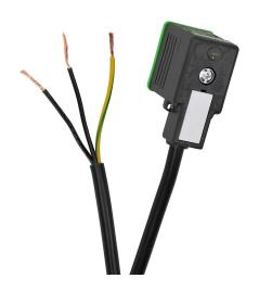
Murrelektronik solenoid valve cable, 10mm DIN 43650 Form B molded connector to 3-wire pigtail, 24 VAC/VDC, 18 AWG, PVC jacket, 16.4ft/5m cable length, surge protection, LED indication.
