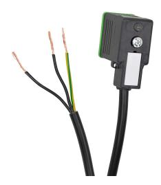
Murrelektronik solenoid valve cable, 10mm DIN 43650 Form B molded connector to 3-wire pigtail, 24 VAC/VDC, 18 AWG, PVC jacket, 9.8ft/3m cable length, surge protection, LED indication.
