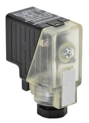
Murrelektronik field wireable solenoid valve connector, 10mm DIN 43650 Form B molded connector, 24 VAC/VDC, 16-12 AWG, accepts cable diameter size 0.24-0.32in, surge protection, LED indication.
