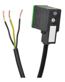
Murrelektronik solenoid valve cable, 10mm DIN 43650 Form B molded connector to 3-wire pigtail, 110 VAC/VDC, 18 AWG, PVC jacket, 16.4ft/5m cable length, surge protection, LED indication.
