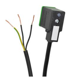
Murrelektronik solenoid valve cable, 10mm DIN 43650 Form B molded connector to 3-wire pigtail, 110 VAC/VDC, 18 AWG, PVC jacket, 9.8ft/3m cable length, surge protection, LED indication.
