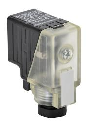
Murrelektronik field wireable solenoid valve connector, 10mm DIN 43650 Form B molded connector, 110 VAC/VDC, 16-12 AWG, accepts cable diameter size 0.24-0.32in, surge protection, LED indication.
