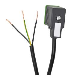
Murrelektronik solenoid valve cable, 10mm DIN 43650 Form B molded connector to 3-wire pigtail, 230 VAC/VDC, 18 AWG, PVC jacket, 16.4ft/5m cable length.
