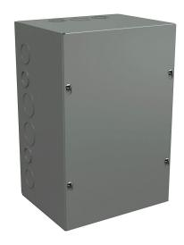
Wiegmann enclosure, NEMA 1, 12 x 8 x 6in (HxWxD), wall mount, with knockouts, carbon steel, ANSI 61 gray, powder coat finish, screw cover.
