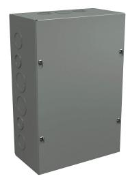
Wiegmann enclosure, NEMA 1, 12 x 8 x 4in (HxWxD), wall mount, with knockouts, carbon steel, ANSI 61 gray, powder coat finish, screw cover.
