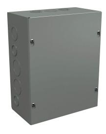
Wiegmann enclosure, NEMA 1, 10 x 8 x 4in (HxWxD), wall mount, with knockouts, carbon steel, ANSI 61 gray, powder coat finish, screw cover.
