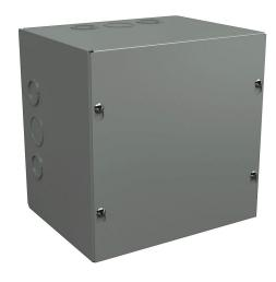
Wiegmann enclosure, NEMA 1, 8 x 8 x 6in (HxWxD), wall mount, with knockouts, carbon steel, ANSI 61 gray, powder coat finish, screw cover.
