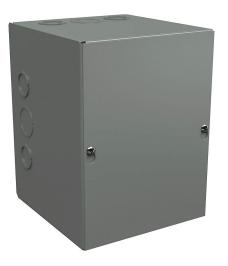
Wiegmann enclosure, NEMA 1, 8 x 6 x 6in (HxWxD), wall mount, with knockouts, carbon steel, ANSI 61 gray, powder coat finish, screw cover.
