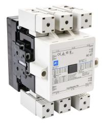
Fuji Electric SC-E7 series IEC contactor, 150A, (3) N.O. power poles, (2) N.O./(2) N.C. auxiliary contacts, 450 VAC (60Hz)/380 VAC (50Hz) coil voltage, low consumption electronic.
