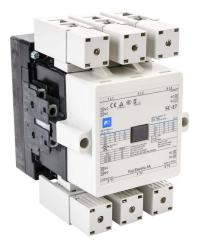
Fuji Electric SC-E7 series IEC contactor, 150A, (3) N.O. power poles, (2) N.O./(2) N.C. auxiliary contacts, 24 VAC/VDC coil voltage, low consumption electronic.
