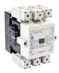
Fuji Electric SC-E7 series IEC contactor, 150A, (3) N.O. power poles, (2) N.O./(2) N.C. auxiliary contacts, 240 VAC (60Hz)/220 VAC (50Hz) coil voltage, low consumption electronic.
