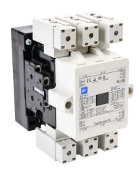
Fuji Electric SC-E6 series IEC contactor, 125A, (3) N.O. power poles, (2) N.O./(2) N.C. auxiliary contacts, 575 VAC (60Hz)/460 VAC (50Hz) coil voltage, low consumption electronic.
