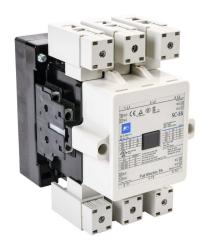
Fuji Electric SC-E6 series IEC contactor, 125A, (3) N.O. power poles, (2) N.O./(2) N.C. auxiliary contacts, 24 VAC/VDC coil voltage, low consumption electronic.
