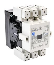
Fuji Electric SC-E6 series IEC contactor, 125A, (3) N.O. power poles, (2) N.O./(2) N.C. auxiliary contacts, 240 VAC (60Hz)/220 VAC (50Hz) coil voltage, low consumption electronic.
