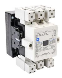
Fuji Electric SC-E6 series IEC contactor, 125A, (3) N.O. power poles, (2) N.O./(2) N.C. auxiliary contacts, 120 VAC (60Hz)/110 VAC (50Hz) coil voltage, low consumption electronic.
