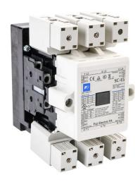
Fuji Electric SC-E5 series IEC contactor, 105A, (3) N.O. power poles, (2) N.O./(2) N.C. auxiliary contacts, 575 VAC (60Hz)/460 VAC (50Hz) coil voltage, low consumption electronic.
