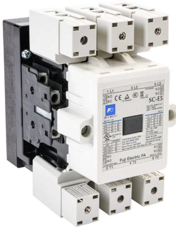
Fuji Electric SC-E5 series IEC contactor, 105A, (3) N.O. power poles, (2) N.O./ (2) N.C. auxiliary contacts, 450 VAC (60Hz)/380 VAC (50Hz) coil voltage, low consumption electronic.
