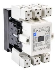
Fuji Electric SC-E5 series IEC contactor, 105A, (3) N.O. power poles, (2) N.O./(2) N.C. auxiliary contacts, 240 VAC (60Hz)/220 VAC (50Hz) coil voltage, low consumption electronic.
