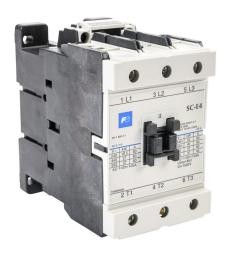
Fuji Electric SC-E4 series IEC contactor, 80A, (3) N.O. power poles, 440-480 VAC (60Hz) coil voltage.
