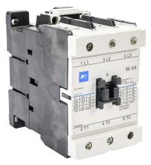
Fuji Electric SC-E4 series IEC contactor, 80A, (3) N.O. power poles, 240 VAC (60Hz)/220 VAC (50Hz) coil voltage.
