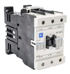
Fuji Electric SC-E3G series IEC contactor, 65A, (3) N.O. power poles, 24 VDC coil voltage.
