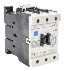
Fuji Electric SC-E3 series IEC contactor, 65A, (3) N.O. power poles, 24 VAC (60Hz) coil voltage.
