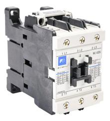
Fuji Electric SC-E2S series IEC contactor, 50A, (3) N.O. power poles, 440-480 VAC (60Hz) coil voltage.
