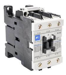
Fuji Electric SC-E2 series IEC contactor, 40A, (3) N.O. power poles, 240 VAC (60Hz)/220 VAC (50Hz) coil voltage.
