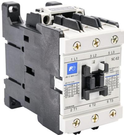
Fuji Electric SC-E2 series IEC contactor, 40A, (3) N.O. power poles, 120 VAC (60Hz)/110 VAC (50Hz) coil voltage.
