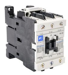
Fuji Electric SC-E1 series IEC contactor, 32A, (3) N.O. power poles, 500-550 VAC (60Hz) coil voltage.
