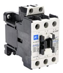
Fuji Electric SC-E05P series IEC contactor, 25A, (3) N.O. power poles, 440-480 VAC (60Hz) coil voltage.
