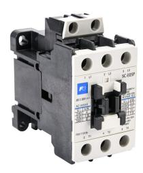
Fuji Electric SC-E05P series IEC contactor, 25A, (3) N.O. power poles, 240 VAC (60Hz)/220 VAC (50Hz) coil voltage.
