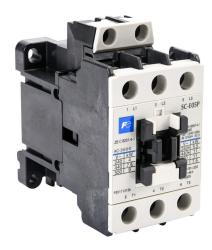
Fuji Electric SC-E05P series IEC contactor, 25A, (3) N.O. power poles, 120 VAC (60Hz)/110 VAC (50Hz) coil voltage.
