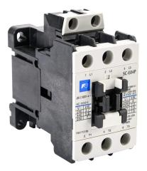
Fuji Electric SC-E04P series IEC contactor, 18A, (3) N.O. power poles, 240 VAC (60Hz)/220 VAC (50Hz) coil voltage.
