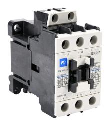
Fuji Electric SC-E04P series IEC contactor, 18A, (3) N.O. power poles, 120 VAC (60Hz)/110 VAC (50Hz) coil voltage.
