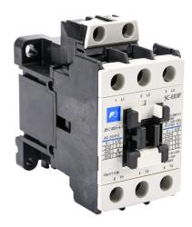
Fuji Electric SC-E03P series IEC contactor, 12A, (3) N.O. power poles, 24 VAC (60Hz) coil voltage.
