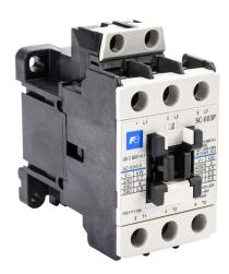
Fuji Electric SC-E03P series IEC contactor, 12A, (3) N.O. power poles, 120 VAC (60Hz)/110 VAC (50Hz) coil voltage.
