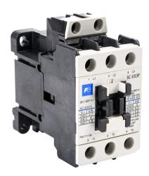
Fuji Electric SC-E03P series IEC contactor, 12A, (3) N.O. power poles, 120 VAC (60Hz)/110 VAC (50Hz) coil voltage.
