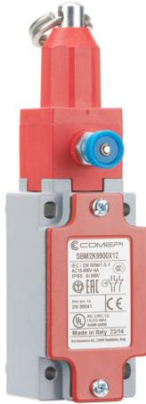
Comepi safety switch, cable-pull interlock, with reset, 25m maximum pull cable length, (2) N.C. safety output(s), (1) N.O. monitoring output(s), die-cast aluminum body, thermoplastic head, (1) 1/2in NPT cable entry.
