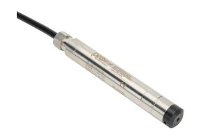
ProSense hydrostatic submersible level transmitter, 0 to 200 psig (461.3ft of water column) sensing range, Output: 1-channel, output current signal range(s) of 4-20 mA, 0.63in diameter housing, shielded and vented 500ft cable.
