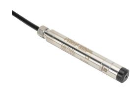
ProSense hydrostatic submersible level transmitter, 0 to 150 psig (346ft of water column) sensing range, Output: 1-channel, output current signal range(s) of 4-20 mA, 0.63in diameter housing, shielded and vented 375ft cable.
