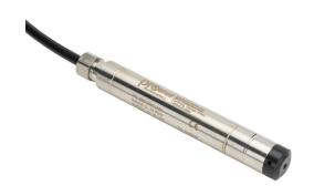
ProSense hydrostatic submersible level transmitter, 0 to 30 psig (69.2ft of water column) sensing range, Output: 1-channel, output current signal range(s) of 4-20 mA, 0.63in diameter housing, shielded and vented 100ft cable.
