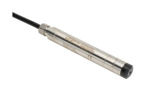
ProSense hydrostatic submersible level transmitter, 0 to 15 psig (34.6ft of water column) sensing range, Output: 1-channel, output current signal range(s) of 4-20 mA, 0.63in diameter housing, shielded and vented 60ft cable.
