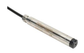
ProSense hydrostatic submersible level transmitter, 0 to 10 psig (23.1ft of water column) sensing range, Output: 1-channel, output current signal range(s) of 4-20 mA, 0.63in diameter housing, shielded and vented 50ft cable.
